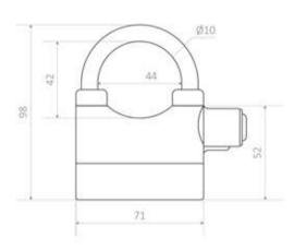
APECS PDZ is a battery-powered padlock with a built-in 110Db siren. It detects shock motion — if the body or shackle are attacked, the siren is activated until manipulations are stopped. Its zinc alloy body and heat processed Hardened Steel shackle ensure it is resilient to cutting and is corrosion resistant. The padlock is extensively used for vehicles, tool boxes, garden sheds, warehouses and many more applications. In addition, the alarm can be disabled when not required.
